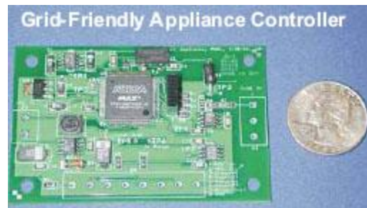
Device to monitor power grid and turn appliances off for a few seconds or minutes in response to overload. Developed by Pacific Northwest National Laboratory. http://www.oe.energy.gov/DocumentsandMedia/Electric_Vision_Document.pdf
